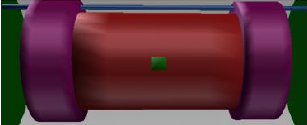
The above diagram features a CAD image of the anticipated rover design while resting in the sabot. The green on the outside of the purple (wheels) represent the bulkheads of the sabot.
