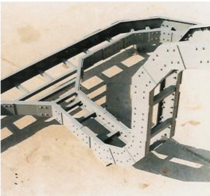
Completed cabletray section prior to shipment to chemical processing plant.
