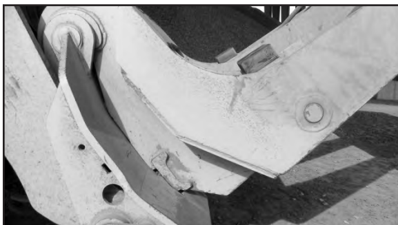
Side View of Subframes and Hooks
