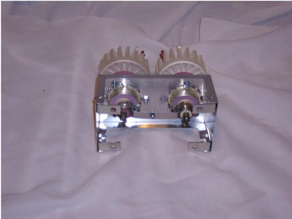
Underside of Tube Socket Assembly
