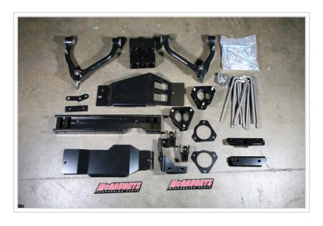
The 4-inch lift kit came with front strut spacers, upper A-arms, a cross member, skid plates and all other hardware needed for the front. For the back end, lift blocks, U-bolts and shock extenders do the trick.
