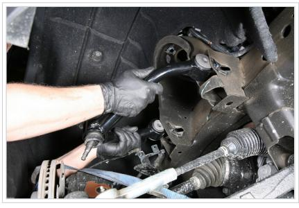
To swap out the A-arms, the cam bolts were unbolted to free them. The new arms were simply placed in and secured with the factory cam bolts.
