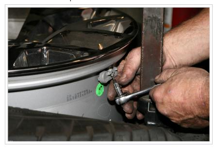
The truck also received an upgraded set of rolling stock. Since the factory wheels have tire pressure sensors, they were marked for their designated corners and taken off so they could be used on the new wheels.
