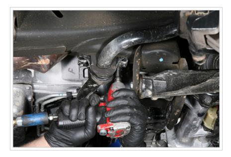
Using a 10mm socket, the sway bar is removed from both sides of the frame.
