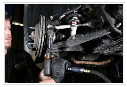
A 21mm socket is used to disconnect the tie rods from the spindles.
