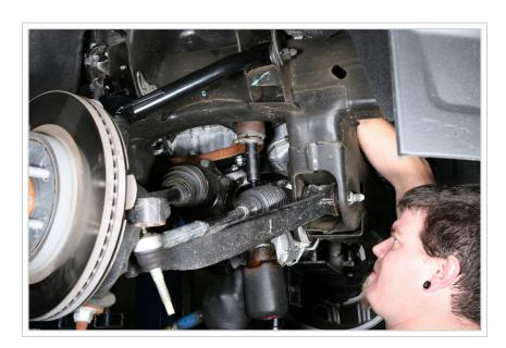
The differential brackets can be reinstalled and the steering can be bolted back on the frame.
