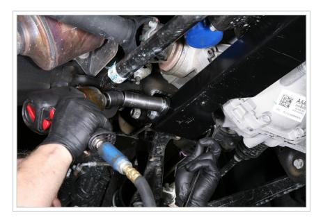
The bracket for the new cross member is bolted between the sway bar mount and the frame. Once in place, the new A-arm bolt can be placed in and tightened down. Note that the CV axle may need to be removed to do so.
