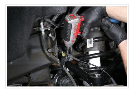
The cool new arms even come with hardware and a mounting location for the ABS sensor wire harness bracket.
