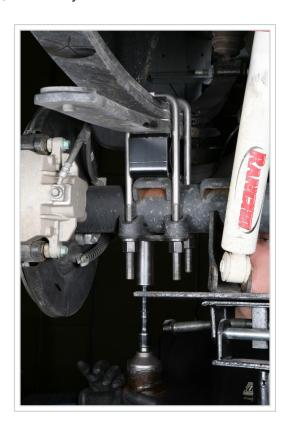
Then the rearend was lowered and the new blocks were dropped in, taller sides towards the rear. The new U-bolts were bolted together to reattach the rearend.
