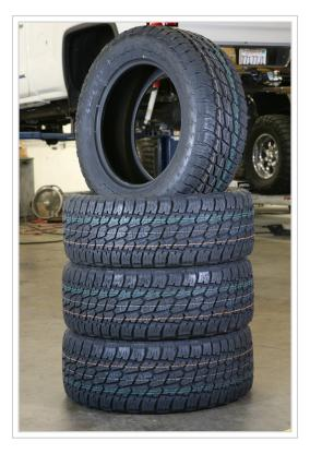
Although this is occasionally used to drive off-road it will mostly be driven on paved roads. For a happy medium we chose Nitto Tires' Terra Grappler, which is an all-terrain light truck radial. It has a nice-looking tread that will grip during all seasons of weather and is designed to minimize road noises. These 305/55R20-sized tires have an overall diameter of 33.19 inches and fit this truck and lift without having any fitment issues.
