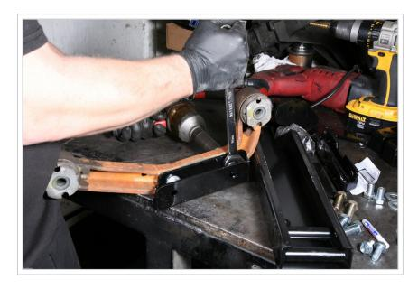
Using a hammer, the factory studs are removed and the drop-down brackets can be installed.
