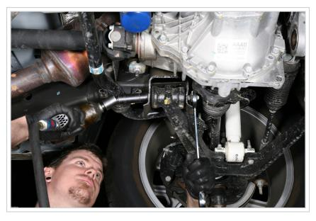
In order to bring the diff down, 3 inches of the frame needs to be cut off where the cross member used to bolt up.
