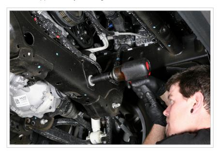
The diff gets mounted lower with the use of a pair of drop-down brackets. To access the passenger side differential, the electronic rack-and-pinion steering needs to be out of the way. To do this, the two passenger side and lower driver's side need to be removed. Then the upper driver's side bolt can be loosened but not removed so the steering can move while remaining attached to the frame.
