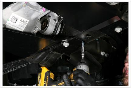
The new skid plates were attached to the front with factory bolts, and the rear is held in place with the supplied ½ x 1-lnch bolts. On the front of the driver's side diff skid plate, two 5/16-inch holes need to be drilled out and two supplied 3/8-inch self-tapping bolts are installed.
