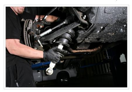
The front strut assembly is unbolted from the frame and lower arm. Then it's removed and set aside for the spacers.
