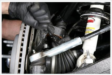
The front started to come together as the tie rods and new upper A-arms were secured to the stock spindles.
