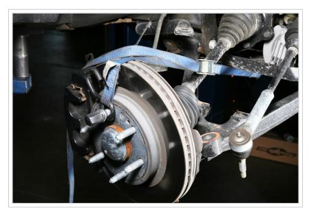
Before the upper arms could be removed, the ball joints were unbolted from the spindles. To minimize stress to the lower ball joints, Chance held the spindles in place with a tie strap connected to the frame.
