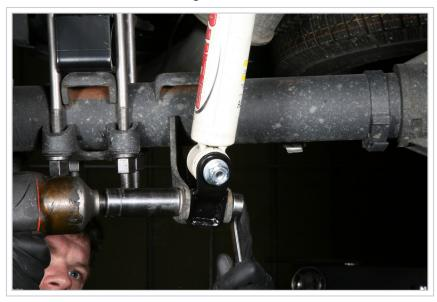
These extenders allow the stock shocks to be used. With the rearend together, the brake line was bolted back on to complete the rear of the installation.
