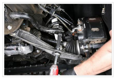
The sway bar and end links are reattached to the lower arms using a 15mm socket and wrench.
