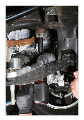
With the diff supported, the differential mounts can be unbolted and removed.
