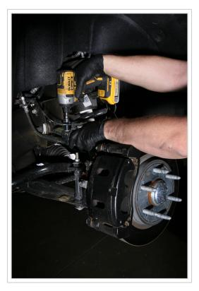
Once you have the truck on a lift or up high on jack stands, you can take off the wheels. The first thing to do on the front is to remove the ABS sensor wire bracket using an impact gun or wrench with a 10mm socket.
