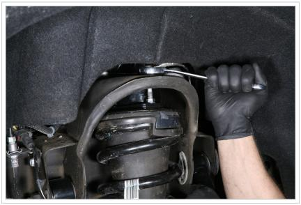
This spacer is mounted to the top of the strut assemblies to make the installation simpler and maintain factory ride quality. Then they're mounted to the truck in the factory locations.
