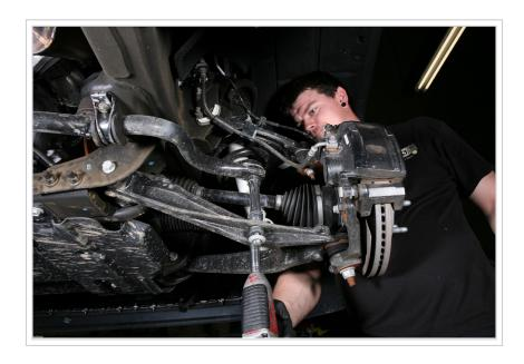
To free the front suspension, the sway bar end links are removed with the use a 15mm socket and wrench.
