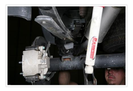
With the rearend supported, the factory U-bolts were removed so that the blocks could be removed.
