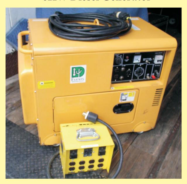
his 6,000+ watt single phase generator is diesel powered. Although not "whisper" quiet it is not construction grade noisy.
