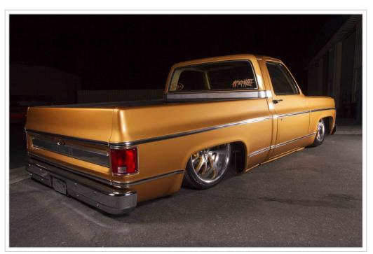
The exterior of the C-10 was kept mostly factory in line with their father's original truck. The trim and bumpers were restored and the rear tailgate insert was polished. A set of One-Piece Products windows was installed, and Carlos Marron made a custom set of stainless steel hood hinges to clear the custom-made wheel tubs.
