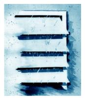
With traditional louvers, "splash" from droplet impact on horizontal surfaces is reentrained in the air stream.
