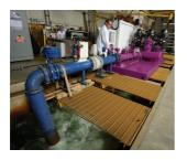
Testing at full flow, vibration, and pressure settings ensure any problems occur at the factory, not at the job site.
