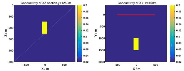
**Figure 1.** Section and top view of the conductivity structure of the 3D model. The red line is projection of the grounded-wire source.
