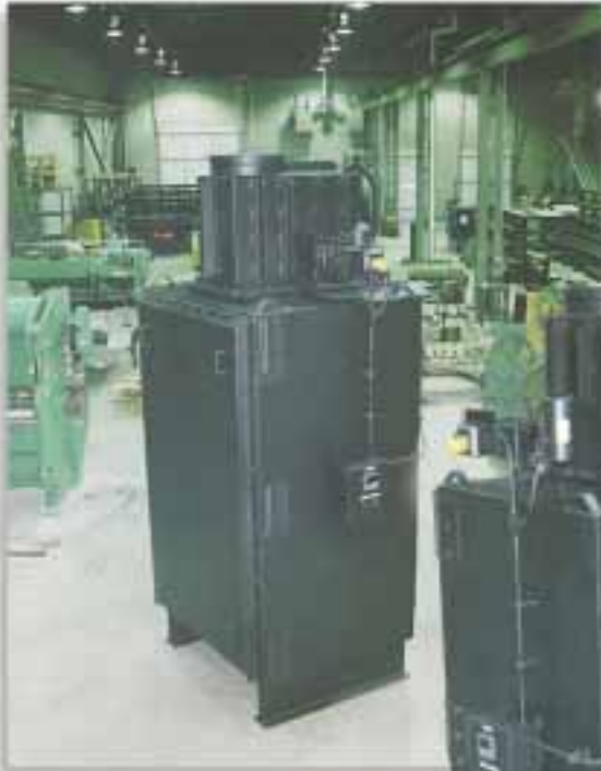
HOSPITAL, Ontario (2) Model HRSR-336B28CSS Recovering Btu from (2) Cummins Wäertsilä CW180, natural gas engines. Reducing each 968°F @ 3,666 SCFM to 339°F. Raising 175 GPM hot water from 195°F to 229°F.
