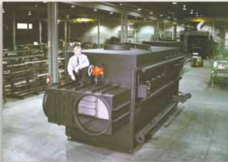
AIRPORT, Detroit, Michigan. (3) Model HRSR-472H28CSS Recovering Btu from (3) Wärtsilä 345G, 5.7MW natural gas engines. Reducing each 698°F @ 18,373 SCFM to 320°F. Raising 175 GPM hot water from 250°F to 350°F.
