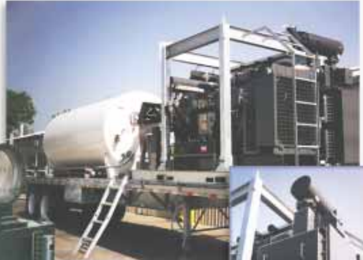
(2) MOBILE TRAILERS, (2) Model HRSR-216826SSS Recovering Btu from a diesel fueled N14 Cummins engine Reducing each 865°F @ 1,188 SCFM to 465°F. Raising 70 GPM 50% Ethylene Glycol from 70°F to 90°F.
