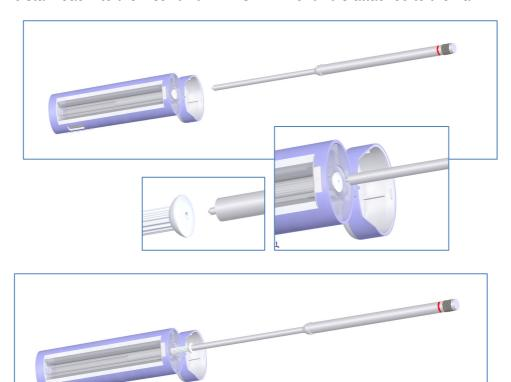
6. Introduce the nail into the hole by sliding the PISTON.
