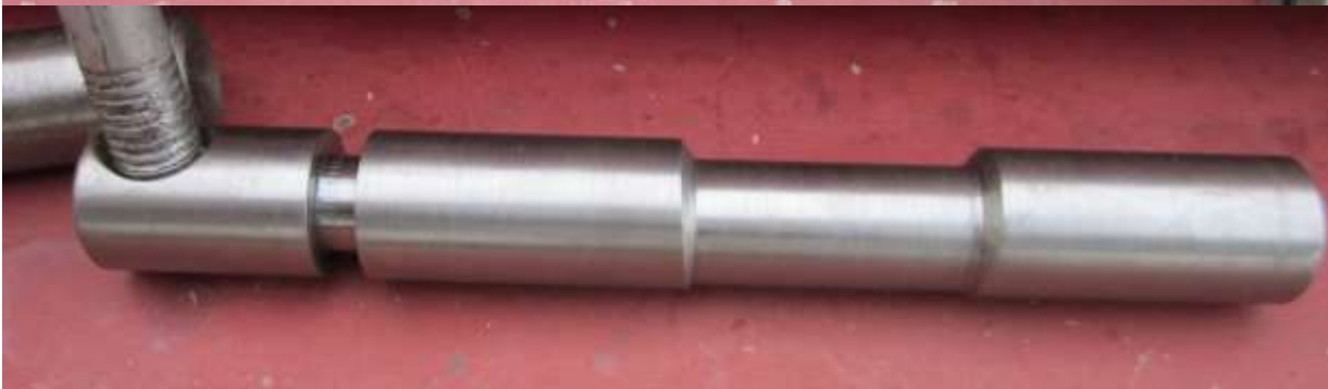
Replacement shaft - courtesy of Bob Monaghan who took his metal lathe and turned the replacement.
