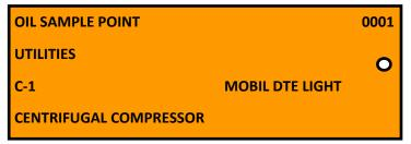
\* An example of our sample point tag that is attached to the sample point location for easy identification
