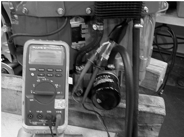
Figure 7-1. Testing AC Output
