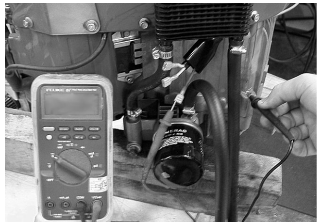
Figure 7-2. Testing DC Output Wire
