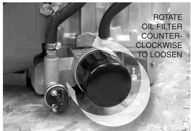
Figure 8-4. Removal of Oil Filter
