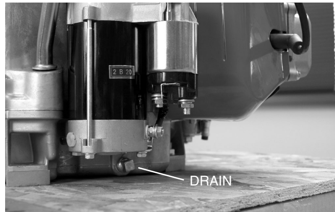
Figure 8-3. Oil Drain Location
