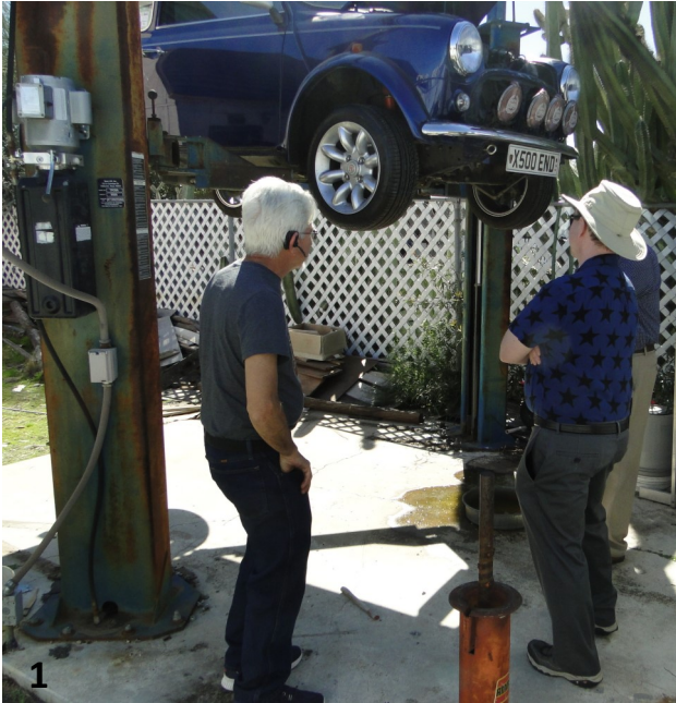
Photos 1 & 2— Having a good look at the under side of a MPI Mini, getting ready to remove the radiator to find out why the fan wasn't working (ended up being a wire that had broken inside the connector).
