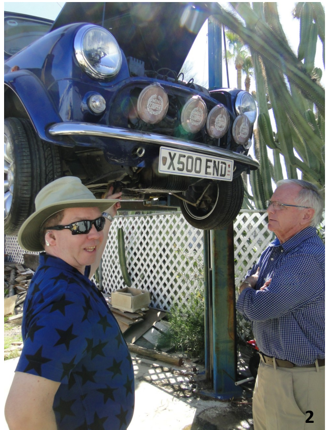
Photos 1 & 2— Having a good look at the under side of a MPI Mini, getting ready to remove the radiator to find out why the fan wasn't working (ended up being a wire that had broken inside the connector).
