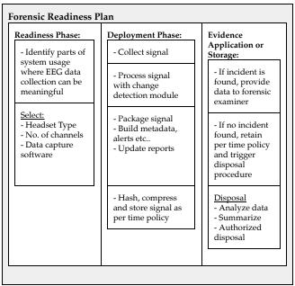
III. Process flow diagram for acquisition, analysis and storage of EEG forensic artifacts
