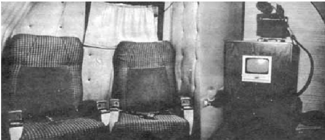
Programming often originates in the studio within the aircraft. Left: Heavily insulated interior blocks out engine and equipment noise. Right: the orthicon camera with its remotely controlled zoom lens and the studio monitor.
