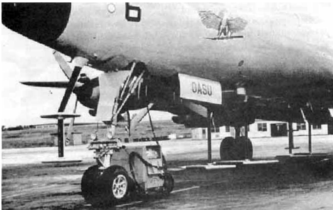
A view of the antenna installation showing a high-band, double-bay, co-linear array mounted forward of the nose wheel and several low-band hayrake antennas mounted in-line on the underside of the fuselage.
