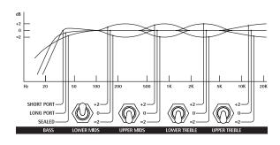
This is the system response graphic that appears on the input/ control panel of the XA Reference. NOTE: The switch settings are for example only. They are not necessarily a recommended setting.
