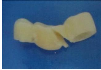
Fracture of reinforced sample
