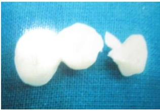
Fracture of unreinforced sample
