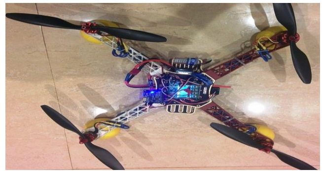
Figure 28: The complete hardware setup of the quadcopter
