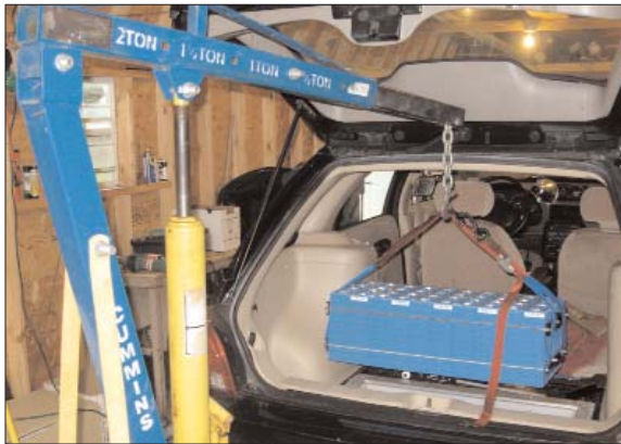
A group of twenty lithium cells being lowered into the Saturn's rear battery box with an engine crane..
