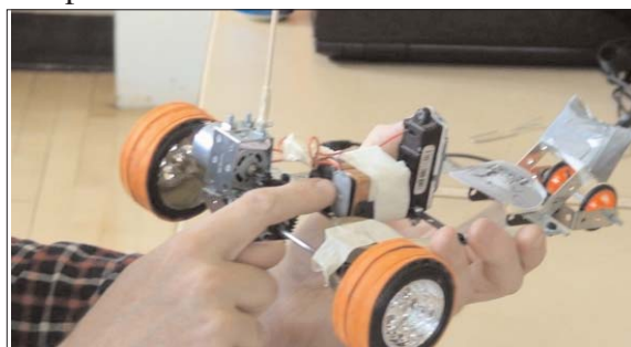
The rear of the car is where the small wheels are close together. The car is somewhat like a tricycle design with the wider spaced drive wheels in the front.
