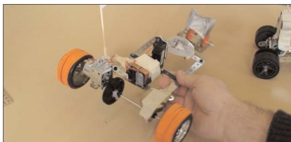
Two nine volt batteries and the switch on top of the motor box housing. Rubber bands on drive wheels for better traction.
