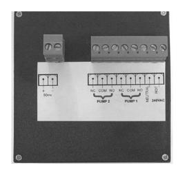
**WARNING:** All board components and circuitry are common to mV signal and must remain isolated from all other circuits and grounds. This is only an issue if board is removed outside protective casing.
