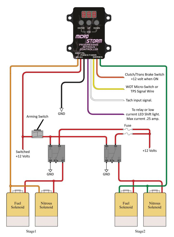
Example showing how to use a relay to convert the Timer Out (ground output) from the MS-001 into a +12 volt output.
