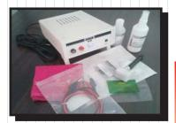
EtchON ME 100", This model is portable manual electrochemical metal etching machine. This model is economical and suitable for small batch production. Etching process is limited only for black/brown marking and suitable for small etching areas.
