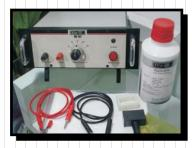
EtchON ME 101", This model is portable manual electrochemical metal etching machine. This model is economical and suitable for medium batch production. Variable Etching Output Voltage for controlling etching Depth and Time, Etching process is limited only for black/brown marking. Suitable for large area etching.
