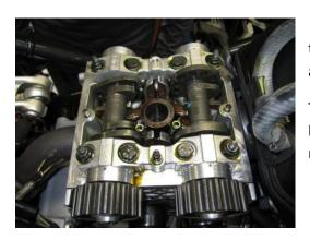
When removing the cam hold-down clamps loosen the inner and then the outer retaining nuts. These nuts are ½ the normal height and it is best to use a 6pt socket.
