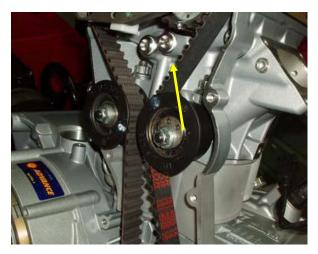
Install the tensioning pulleys and the Fuji nuts, but don't tighten them yet.
