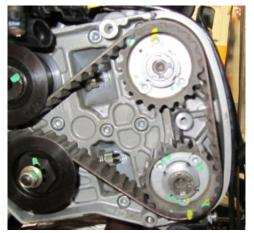
The yellow marks pictured on this horizontal cylinder are made on the pulleys where the valve cover gasket sets on the cylinder head. The three previous pictures show the pulley alignment at the "home" position . The markings will be necessary for reassembly when the belts have to be removed for shim (or belt) changing.
