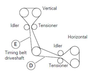
Use 19 ft lbs of torque on the belt tensioning nuts
