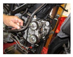
Use a punch and gently tap on the pulley to loosen the cam/cam retainers so the cam shafts can be removed.
