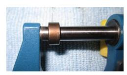
Close the micrometer. Do not over tighten. Press the "zero" button to set the reading to 0.00. Open the micrometer and place the shim on the stationary shaft of the micrometer, with the flat side towards the fixed portion of the micrometer. Measure the opening shim and record the measurement in column D of the worksheet. Determine the size of the replacement shim by adding column C to column D and record this number in column E. The number in column E is the ideal shim size to
