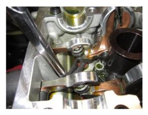
With the cam removed, the opening shim will lift off of the valve. Hold the opening rocker out of the way. Use a magnet or needle nose pliers to remove the opening shim. If replacing more than one opening shim put it in a marked container (plastic bag, egg crate, etc. so it doesn't get mixed up with other shims.
