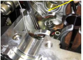
If a closing shim requires replacement to bring the valve clearance into specification the opening shim will have to be removed from the valve. Remove the opening shim and set it aside, marking the shim's location for reassembly.
