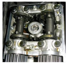
This is what you will see when the cover is removed. Confusing at first, but after a few minutes it all makes sense. No black magic or voodoo is involved, just beautifully machined surfaces designed for a purpose. Note the opening cam lobes (the smaller, inner cam lobes) are pointing "up" which indicates the valves are in the "rest" position and ready for measurement.
