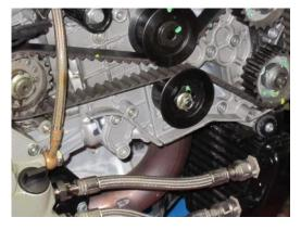
Loosening the tensioning pulley is accomplished by loosening the Fuji nut and rotating the tensioning pulley clockwise (away from the cam drive gears). Loosen the nut and remove the tensioning pulley from its mounting stud on the cylinder head. Removing the tensioning pulley facilitates belt removal/installation. Label the tensioning pulley (horizontal or vertical).
