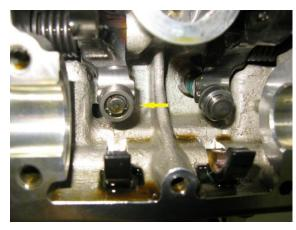
Here is the horizontal cylinder with the cams removed. You can see the opening shim has been removed from the valve on the left and the closing shim is accessible.
