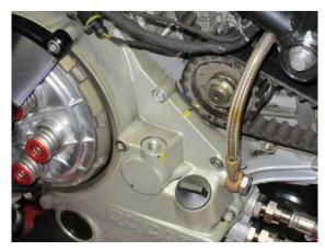
With the belt covers removed check alignment on the belts and pulleys. The intermediate shaft drives the cam belts. There is a mark (dimple)on the pulley and a mark on the engine case. At TDC of the horizontal cylinder, the marks will align. Use the paint pen to mark this alignment. Slight rotation of the engine forward/back may be necessary to locate TDC at this point.
