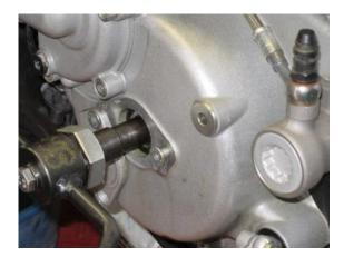
Once the spark plugs are removed, the engine turning tool can be installed. Remove the cover on the left side of the engine and install the engine turning tool onto the end of the crankshaft. Note: the tangs on the engine turning tool fit neatly into indents on the crank shaft. Tighten the bolt to snug and the engine is ready to turn counter clockwise (CCW) into the correct position(s) for valve clearance checking.
