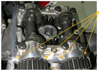
Put gasket sealant on the mating corners where the cam retainers meet the flat surface of the cylinder head/valve cover for sealing. Torque in 2 stages to 7ft lbs.
