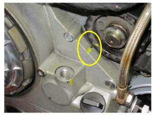
Align the marks on the intermediate shaft and the engine cover.
