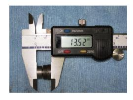
Add column H to column I to find j: the size of the closing shim to bring the clearance into specification. The closing shims can be sanded into the exact size with 400 wet/dry sandpaper if one of the standard sizes doesn't
