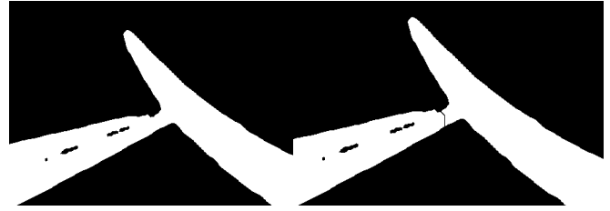
Fig. 4. Sequence illustrating the effect of segmenting blobs through watershed segmentation. On the left image, blobs are initially connected. On the right image, watershed segmentation is applied to blob.
