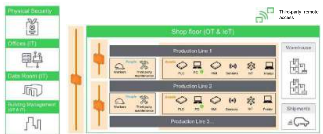
Figure 1: Network segmentation to separate IT and OT environments
