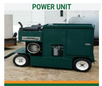
Provides power to the Crawler through a 23hp LPG powered Kubota engine that can also be custom designed to run on a 25hp electric motor.
