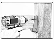
STEP #4 - Locate 2x4 railing on post and use 4 each screws to attach railing to post.
