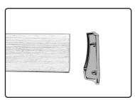
STEP #2 - Place 2x4 into railing connector.
