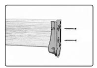
STEP #3 - Use 2 each screws to attach railing connector to 2x4. (Pre-drill holes if desired)
