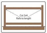
STEP #1 - Measure distance between posts, subtract 1/2" from overall length to account for 1/4" railing connector thickness. Cut 2x4s to create top and bottom rails.
