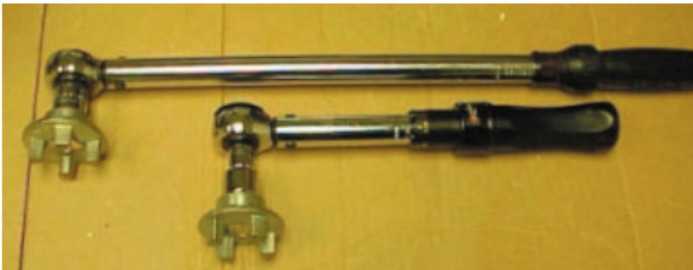
Top: Craftsman (Sears) 210 N-m Bottom: Performance Tool Brand 29 N-m
