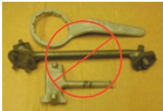
Wrenches suitable to open and re-close drums for in house use. Cannot be used to close drums for shipment of hazardous materials.
