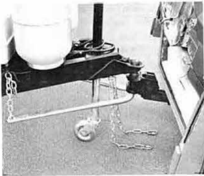
3. Raise trailer and car, attach bars.
