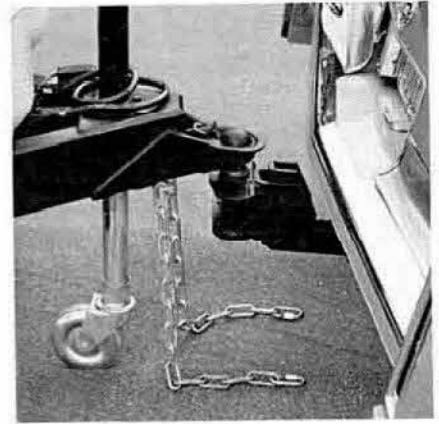
2. Lower trailer, insert safety pin.
