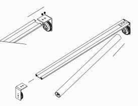
For installation, mount brackets to mounting surface and snap headrail into brackets.
