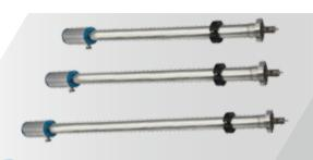
For application that require combined rotary and linear movement, Magnetic Transfer Rods can be used. These devices use a magnetic coupling to drive both linear and rotary movement to the shaft. The shaft is mounted with bearings that allow it to move in both a linear and rotational manner. The MTA is a completely enclosed welded structure. The tip of the vacuum side is special designed so that sample carrying mechanism or other custom devices can be mounted.
