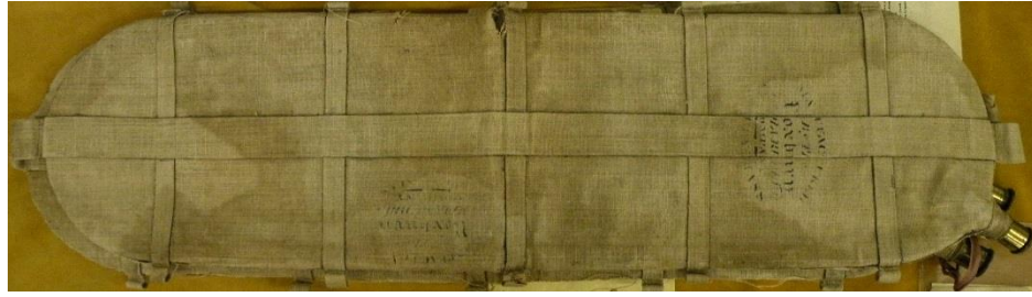
One of the three pontons that make up the model. This ponton is stamped by the manufacture on one side and signed by the inventor on the other.
