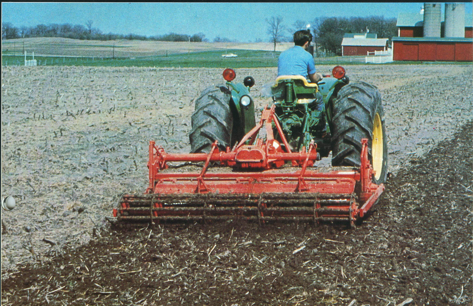
Model E-80 shown above is equipped with an optional crumble roller.
