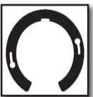
This ring is designed to transform any standard five gallon bucket into a core catcher and will catch up to 8" cores!
