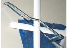
Firstly, cut the one on the top, and make a mark on the one under. Secondly, gently put the one that was under and put it on the top. Use the mark done on the PVC to cut it. Then use your hard nylon hammer to push the PVC ends to join them. When done, it is time to cut the extra graphic with a cutter.
