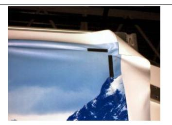
Start positioning and putting in place, starting from the top, the graphic using 5"-6" long TS79W segments. Important: Only use a hard nylon
