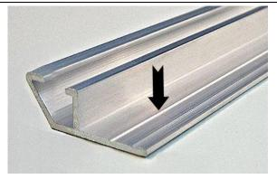
After having measured, miter the corners, and cut the TS23 extrusions to the desired length, to fabricate the frame, screw the extrusions to the trucks, or trailers sides (with <u>one metal screw every 20")</u> at the place indicated by the arrow on the photo. Then start positioning, fixing and installing the printed graphic material (See how hereafter)
