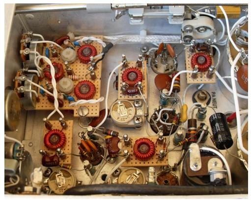
Toroids used in the IF and RF circuits of the Vintage SSB Special transmitter. Ceramic trimmers are used to resonate the ones used in tuned circuits.
