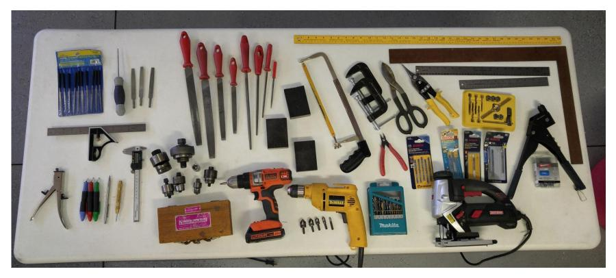
These are all pretty common tools, and most are not expensive. I did collect an assortment of chassis punches, which proved invaluable for making holes for tube sockets and meters. Of course you can drill and file out those big holes, but it will take a few extra days and they might be almost round when you're done!
