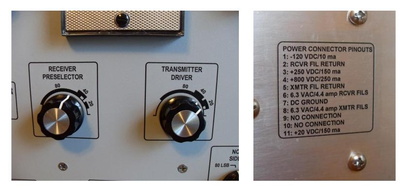
These labels were made with water slide decals printed on Papilio stock with an HP laser printer. The labels were designed using Microsoft Visio software. The front panel was oversprayed with clear matte finish from a rattle can. The chassis label was brushed with polyurethane semi-gloss.
