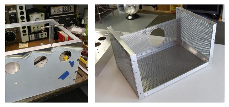
These pictures show how the cabinet used for the 2X813 linear was made. The same techniques were used for the Octal Tri-Bander and PSSU cabinets.
