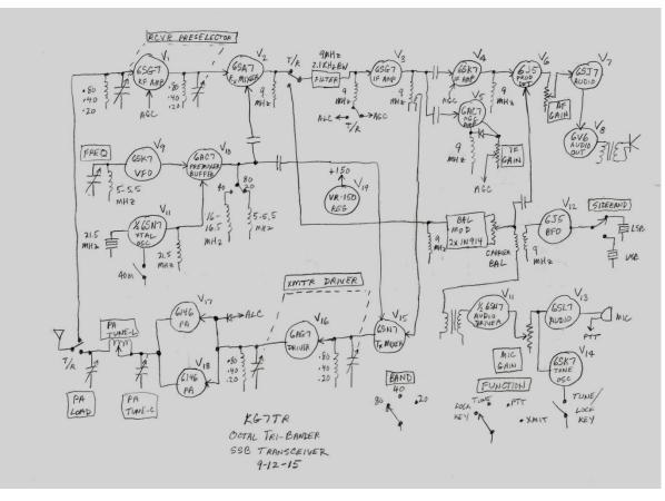
If the project will be complex, I sketch out a block diagram of the major parts and circuits. This is the rough diagram I used for the Octal Tri-Bander.
