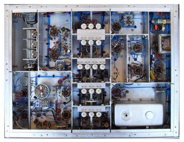
Bottom view. 4" high chassis allows ARC-5 VFO components to be mounted upside down for a more useable location of the main frequency knob.
