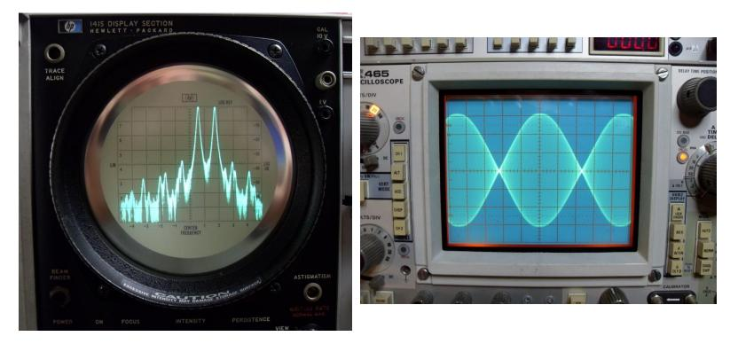
Two-tone RF output at 40 watts PEP. This radio produces very clean SSB.
