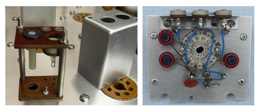
Coil construction used in the Octal Tri-Bander transceiver. At left, coil can and internal parts are from an airborne transceiver. Fiberglass peg is pushed into rubber grommet. Toroid will be epoxied to peg and ancillary components mounted on standoffs on bottom fiber base. At right is shown a removable bandswitch section. Fiberglass pegs pushed into a grommet are used here as well. In both cases, diameter of the peg is increased with masking tape to make a snug fit of the toroid.
