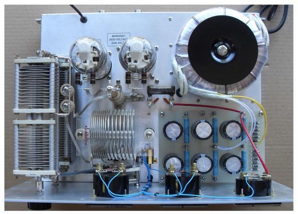
An Antek 800VA toroid feeds a voltage doubler that provides about 2,250 VDC no load. The PA coil is an Illumitronic pi dux 2408D4 pruned for 80, 40 and 20 meters. Bandswitch is a Radio Switch unit. Braided wire for RF wiring allows flexing as chassis is handled.
