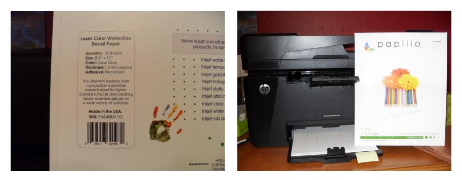
The decal stock is very inexpensive and is available from papilio.com. They make decal stock for inkjet and laser printers. With an inkjet you have to spray Krylon or similar on the sheet to keep water from dissolving the ink. But you can do color with an inkjet printer. With laser stock no overspray is required. If you have access to a color laser printer, that will make color decals too.
