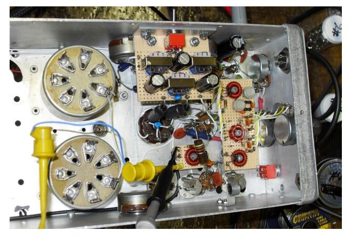
Here the audio and 9MHz SSB generator circuits of the 80m Cheap 'N Easy II are being tested. No sense going any further until this stuff is working!
