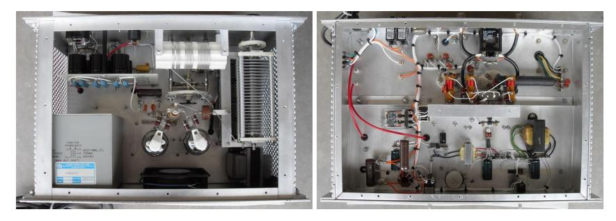
Voltage doubler delivers about 2,700 VDC no load. PA coil is wound on a form from a TU-5 unit. Bandswitch is heavy duty unit made by Radio Switch Corp. Plate transformer was a NOS military unit from Surplus Sales, but they are now out of stock. Input is tuned by bandswitched pi-net circuits. A 3 second soft start circuit is used in the HV supply. The filament choke was made from an Amidon kit.
