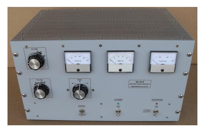
This linear was built to go with the Octal Tri-Bander. I always liked the look and feel of an 813. This amplifier uses a pair of them in grounded grid. A lot of the design is similar to my HB-600 linear. NOS Triplett meters monitor grid mA, plate mA, and plate VDC.
