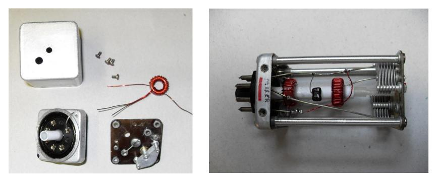
Examples of ways to make a shielded coil using a coil can from an ARC-5 receiver. Most of the Octalmania coils were made this way. Note that the original air variables are used to resonate the circuit.
