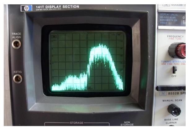
"White noise" audio input experiment verifies 2.5 KHz bandwidth of 8 pole solid state Butterworth filters
