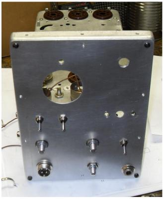
When building a radio on a Command transmitter chassis, I totally strip and clean it first. Then I build from there. These pictures show the 80m Cheap 'N Easy II under construction. Note the new front panel overlay.
