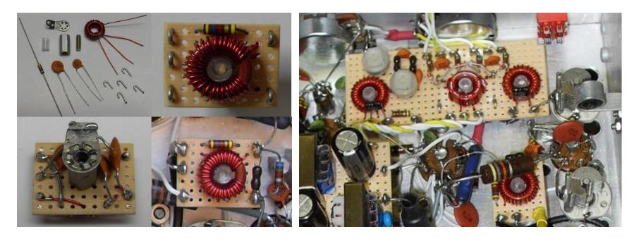
Perf board and threaded spacers provide one way to mount toroids. You can also mount ancillary parts on the board. Simple loops of tinned #18 wire can be pushed into the board and used as terminals for external connections.
