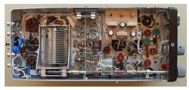
Inexpensive transistor audio transformers from Mouser are used in place of the unobtanium surplus units in the original W2EWL design.
