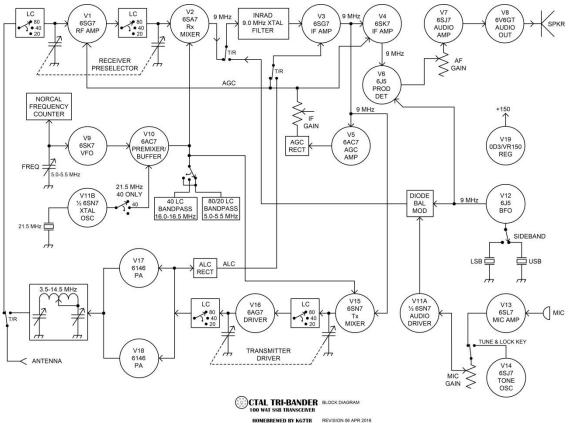
Block Diagram. I actually wired and tested the whole radio from a penciled version of this, and kept rough schematic notes where necessary. When the radio was finished and working right I drew up the final, detailed schematics.
