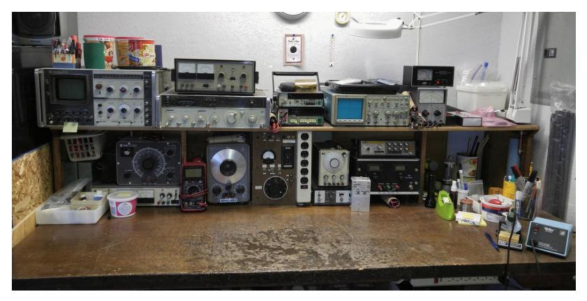
Decent test equipment really helps. For an SSB transmitter, essential are a wideband scope, two-tone audio oscillator and spectrum analyzer. For a receiver a good signal generator is a must. You need a frequency counter for either. The Heathkit lab power supply is useful for breadboard and element testing.
