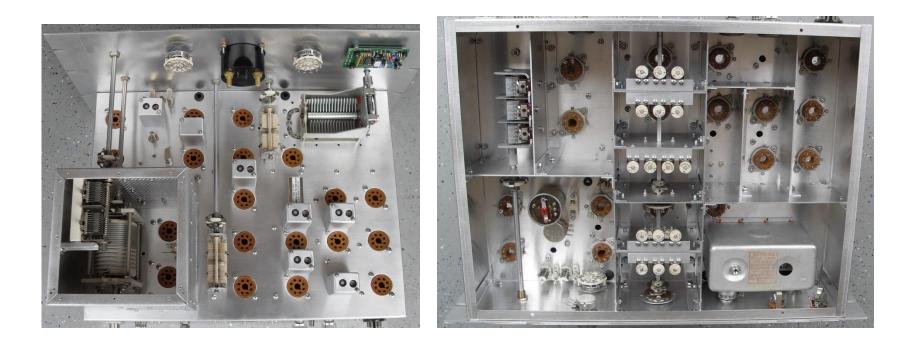
Sheet metal work done, ready to start wiring. A lot of thought went into laying everything out. Transmitter circuits are on the left and receiver circuits are on the right. Bandswitched circuits are smack in the middle.
