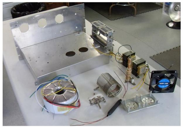
Layout is mostly about making sure RF paths are short, the front panel is functional and pleasing in appearance, there are no interferences, and parts can be removed and replaced if necessary. This is the 2X813 linear under construction.
