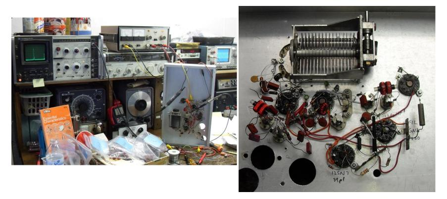
When I have to use a circuit I've never tried before and there is risk of a lot of tweaking, I breadboard it first on an old junk chassis. This is the breadboard used to develop the new 40m buffer/premixer circuit used in the Octal Tri-Bander.
