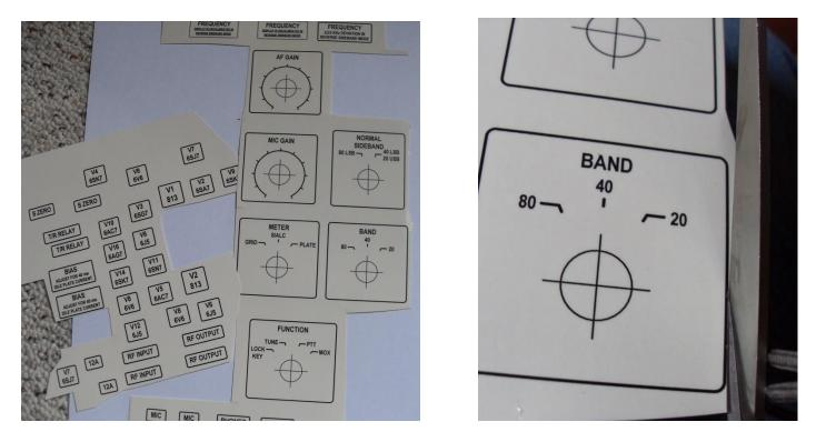
A good pair of sharp scissors is used to cut out each decal. Putting a box around each decal makes the transition on the panel less perceptible, and provides a way to line up the label parallel or perpendicular to an edge.
