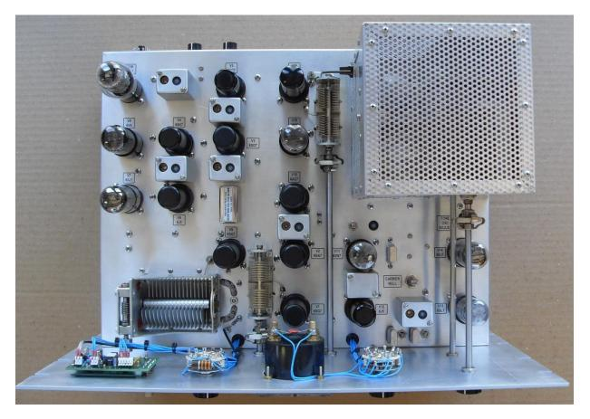
Top view of completed radio. Receiver preselector and transmitter driver use separate tuned circuits, unlike most tube type transceivers.
