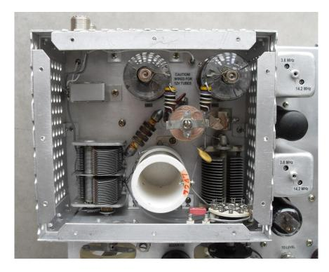
Inside PA Cage. Pair of 6883s (12 volt version of 6146) deliver 100 watts PEP. Coil wound on ARC-5 PA form. Antenna relay is at upper left.
