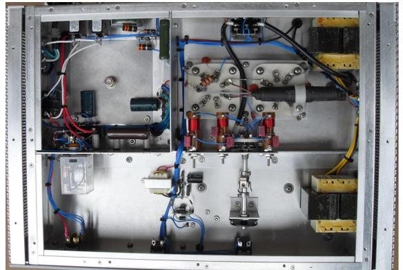
Bandswitched, tuned input circuits are used. Two 5 volt, 10 amp control transformers are connected in series to provide filament voltage for the 813s. The filament choke is from an Amidon kit. The chassis is braced with angle stock and a right angle shield to provide a robust foundation for the toroid power transformer.
