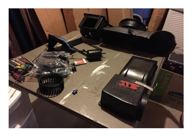
I installed the new seals using a spray adhesive. Weatherstrip adhesive will also work. The factory heater core was a brass/copper unit. Brass/copper replacements are still available, but at twice the price of an aluminum core. The aluminum heater cores are just as durable and actually transfer heat a little better.
