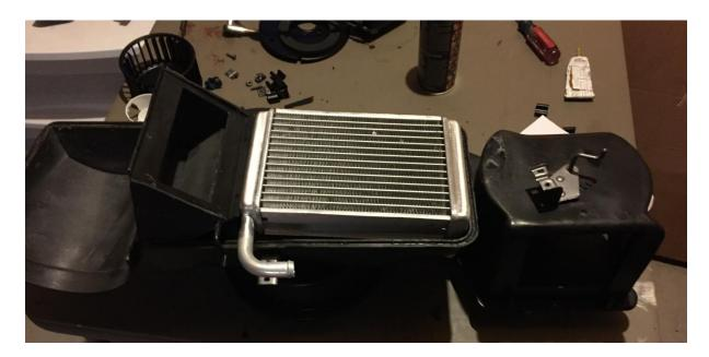
Here's where that 3M strip caulk from part 1 of the article comes in handy. The seal kit comes with a new seal for every other area, but the area between the blower motor and the heater box requires strip caulk. I tested the original blower motor with a car battery and found it was still working just great. Replacement motors are available, but you'd be hard pressed to find one made as well as they were back in the 1960's.
