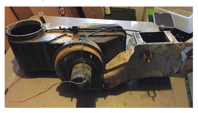
Inside, all the was metal was rusted. Most of the seals were disintegrating.
