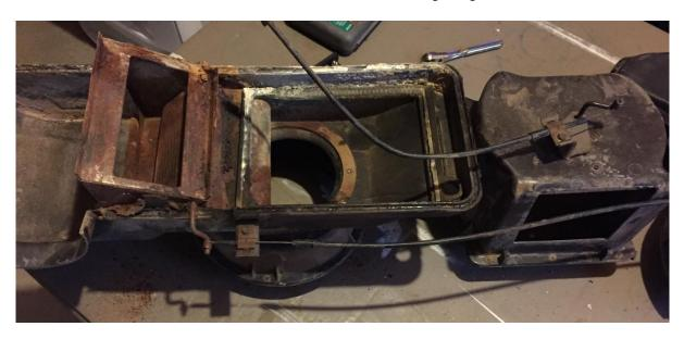
I cleaned all the metal parts in the blasting cabinet and scrubbed away all the grime with warm, soapy water. To replicate the factory look, the fiberglass box should be bead blasted and reshot with clear. I simply painted my box with Duplicolor trim paint. The metal parts got a coat of self-etching primer and two coats of trim paint. I think it turned out pretty spiffy.
