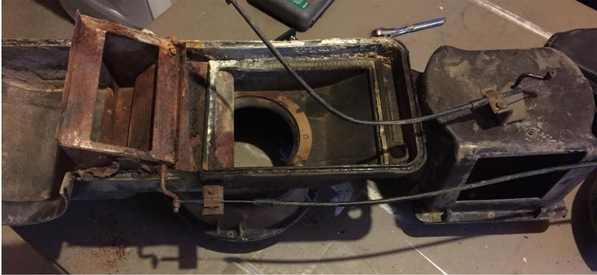
I cleaned all the metal parts in the blasting cabinet and scrubbed away all the grime with warm, soapy water. To replicate the factory look, the fiberglass box should be bead blasted and reshot with clear. I simply painted my box with Duplicolor trim paint. The metal parts got a coat of self-etching primer and two coats of trim paint. I think it turned out pretty spiffy.
