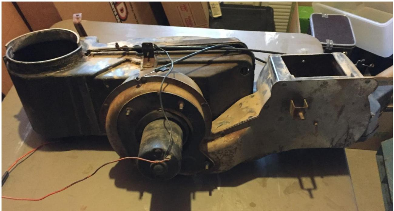
Inside, all the was metal was rusted. Most of the seals were disintegrating.
