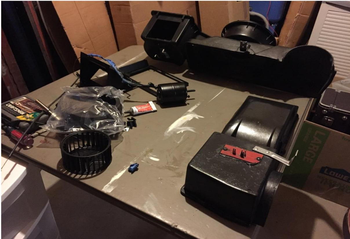
I installed the new seals using a spray adhesive. Weatherstrip adhesive will also work. The factory heater core was a brass/copper unit. Brass/copper replacements are still available, but at twice the price of an aluminum core. The aluminum heater cores are just as durable and actually transfer heat a little better.
