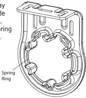
Press the motor into the bracket, spring ring will open slightly allowing the motor to enter and then the spring will close, firmly locking the motor to the bracket. Ensure the spring ring is inside the groove of the bracket and the motor.
