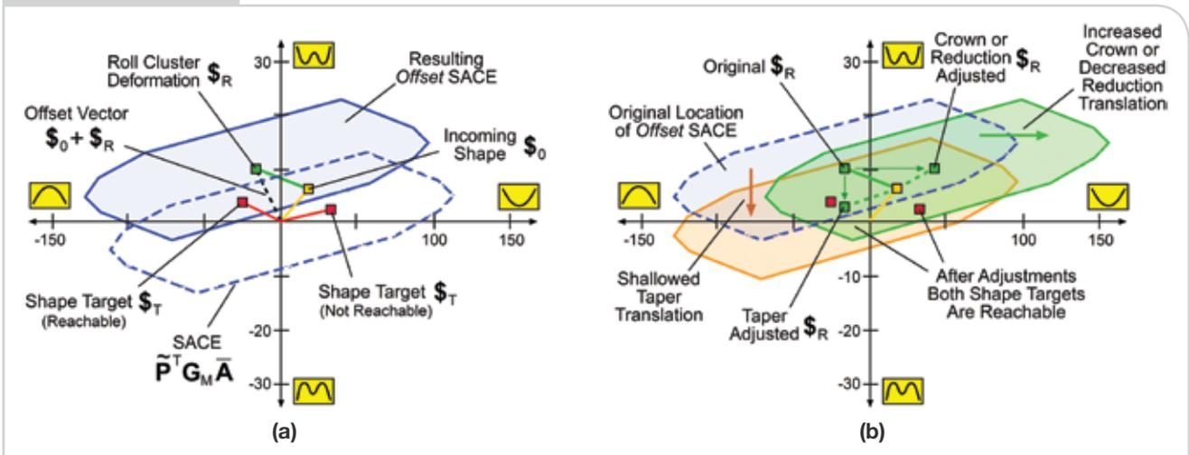
Diagrams showing the formation of the *Offset SACE* (a), and how changes to the pass scheduled reductions or mill setup induce a shift in the *Offset SACE* (b).
