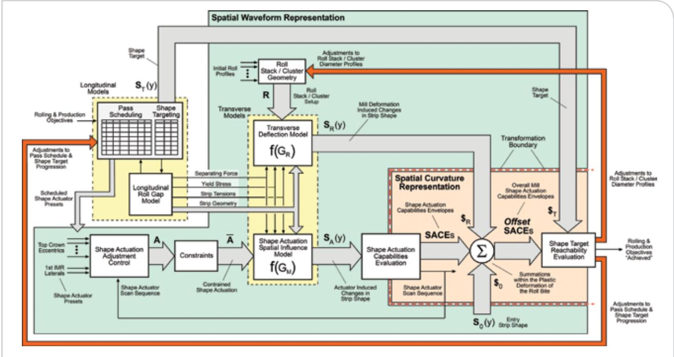
Block diagram illustration of the procedural design sequence and information flow.
