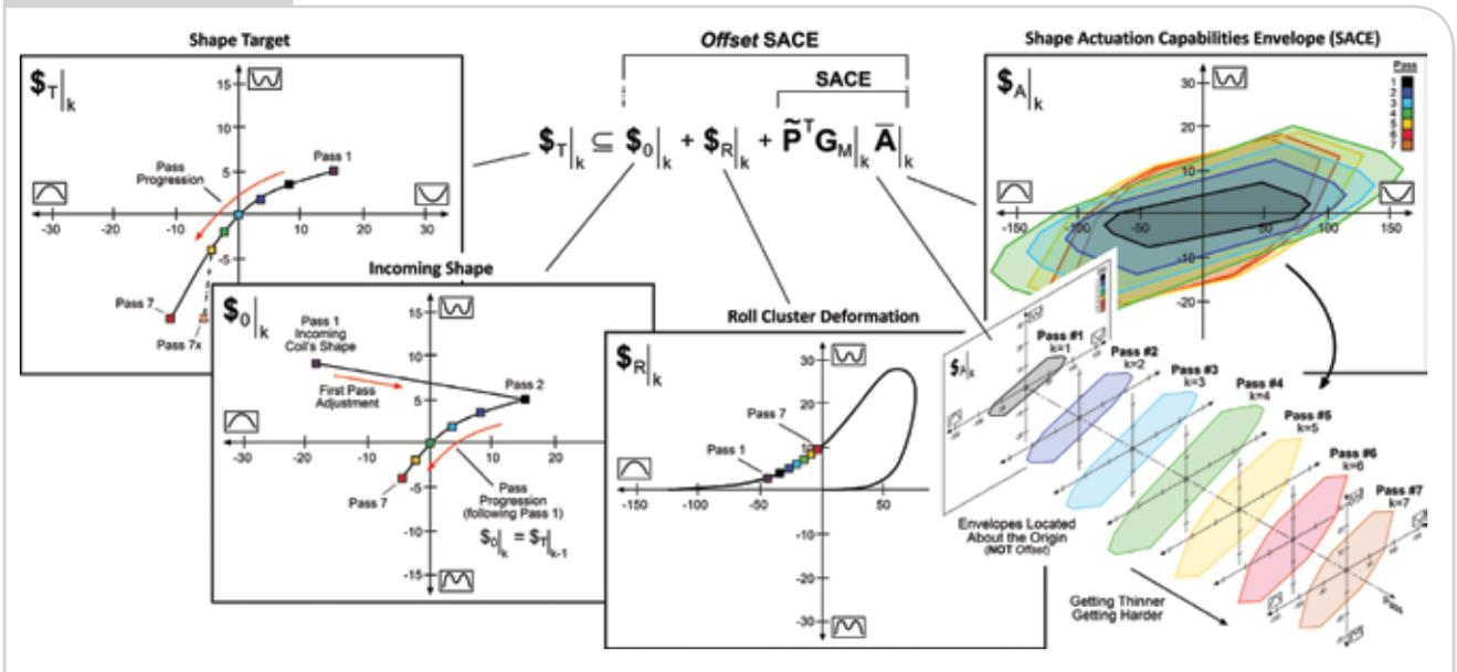
Diagrams showing the focal point of the design process and the pass-to-pass components forming the *Offset SACE*.
