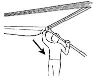
Release the snap stud of the main arm and lower the awning to its lowest position.
