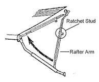
Standing under the awning, release the rafter arm by pulling outward on the cap of the ratchet stud located on the upper portion of the arm. Extend the arm and place the claw over the shaft of the roller.
