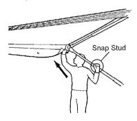
Raise the awning to the desired height by releasing the snap stud on the main arm and pushing up and outward on the roller assembly.
