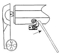
Insert the pull rod into the travel latch loop and rotate open
