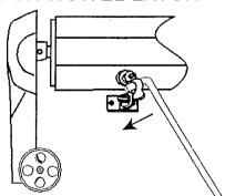
Insert the pull rod into the travel latch loop and twist shut.
