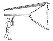
Insert the pull rod in the loop of the center control strap and unroll the awning to the desired extension.
