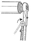
Swing the clamp wheel assembly toward the hardware and fit into place. Then turn the clamp wheel clockwise to tighten.
