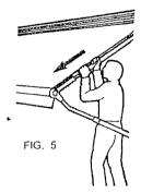
Set the spring tension of the rafter arm by grasping the lower arm and pushing firmly down in the direction of the arrow as shown, until the ratchet stud engages to lock the arm open. (Listen for click)
