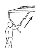
Face the awning and hold the end of the center strap then push the roller up briskly with a rolling motion until you feel the spring take over. Control the speed by holding the center strap until all but 6 inches of the fabric has been rolled up. Release the strap and let the awning roll freely the rest of the way.
