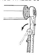
Turn the clamp wheel counter clockwise and swing the assembly toward the center to free the hardware
