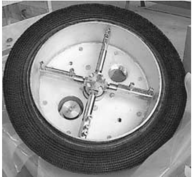
Fig. 5. Vacuum shroud with 10-jet spray bar configuration.
