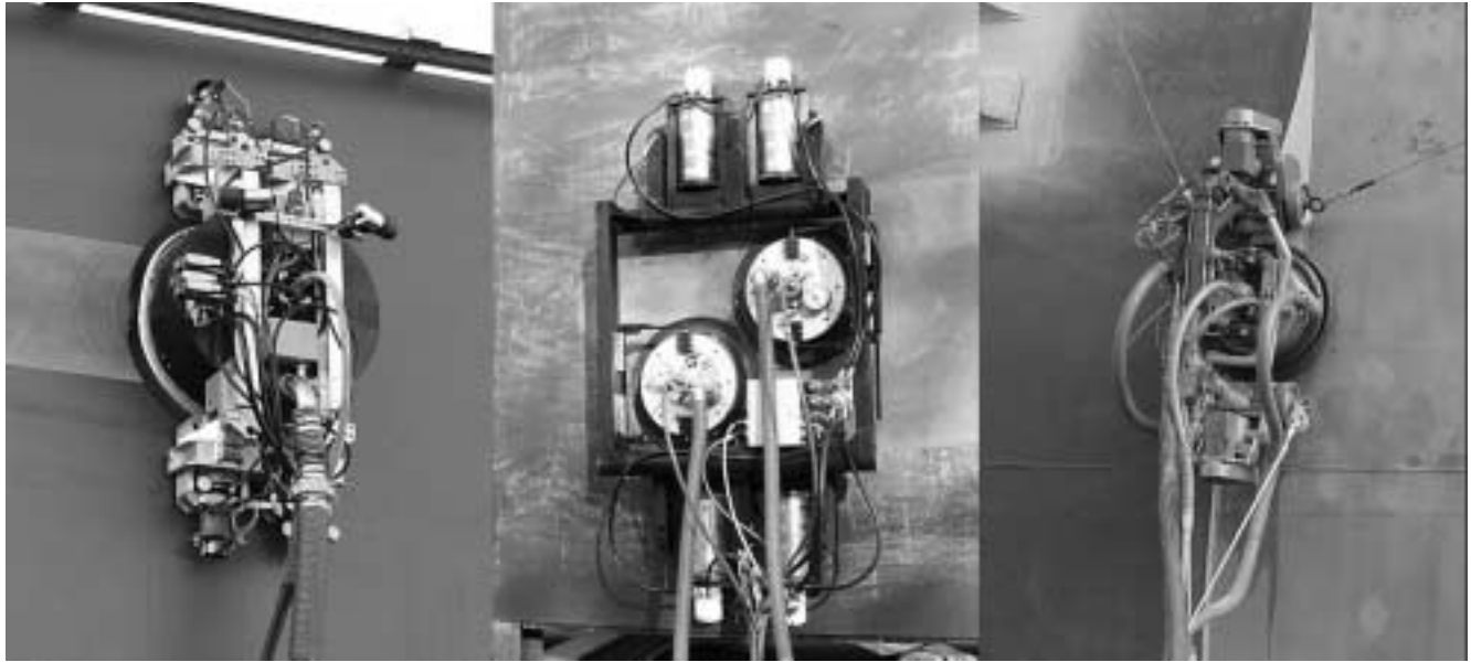
Fig. 3. The three versions of the NREC-UltraStrip Systems robot chronologically from left to right. The wires in the right-hand image are passive inertial safety reels to catch the robot in the event of a fall.
