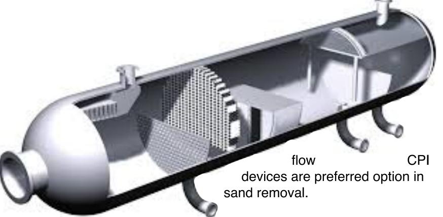
The plate coalescer are simple devices that have no moving parts and do not require power. Steady flow rates with oil concentrations up to 3000 ppm and limited amount of solids are the favorable operation conditions. Emulsified flow streams and oil droplets below 30 µm significantly reduce the efficiency of this equipment type.
