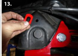
**11.** There is a small hole in the factory 4-link mount. This hole must be drilled out to 1/2". Once drilled out, use the provided shim to fill the void between the new bracket and the factory mount. Use the provided 1/2" x 1-1/2" bolt and tighten down. (pic 11-14)
