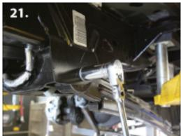
**20.** Remove the factory radius arms, using a 27mm socket on the upper axle bolt and a 24mm socket with a 27mm wrench on the lower axle bolt. (pic 20) Use a 27mm socket on the frame side to remove the radius arms. (pic 21)
