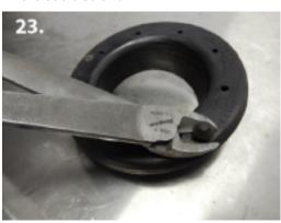
**22.** Before installing the new supplied lift coils, be sure to trim the protrusion off the factory coil insulators as shown. (pic 23)
