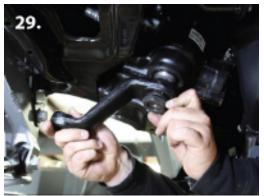
**25.** Install new drop pitman arm, DC602. Apply the supplied red thread locker to the factory pitman arm retention nut and tighten to factory specs. (pic 29) **NOTE: Check and re-torque this nut after the first 500 miles fo driving.** 26. Loosen the drag link adjuster lock nuts. Turn the adjuster until the drag link is free.
