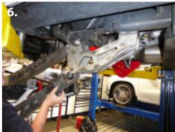
**3.** While holding the upper arm in place, install the 4-link drop down bracket using the provided hardware. (pic 4) **4.** Install the lower 4-link arm onto the lower axle mount using the factory hardware. Then, install the rear of the lower arm into the drop down bracket using the provided hardware. (pic 5-6)
