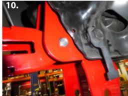
10. Use the provided 20mm x 140mm bolt to install your factory lower arms into the new brackets.
