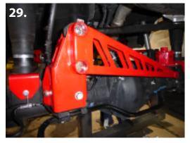
**27.** All hardware for the track bar bracket and braces should now be tightened. Finished, it should look like this. (pic 28-29)
