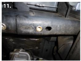
**6.** Once the hole is drilled out, install the provided rivet nut. Use the provided rivet nut tool with a 3/4" socket and IMPAC tool to crimp the rivet nut inside the frame. (pic 9-11)
