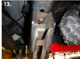
7. Reinstall the 4-link drop down mount to the frame using the provided hardware. Next, reinstall the upper and lower arms. (pic 12-13)
