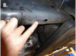
**5.** Make sure new 4-link drop down bracket is pushed all the way against the bottom of the frame. Use the bracket as a locator to drill a 1/2" hole. Next, remove the 4-link mount from the frame so that you can drill the hole out to 11/16". (pic 7-8)
