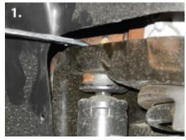
With the parking brake set and wheel chocks behind the rear tires, use a jack to lift the front of the vehicle and place jack stands under the frame on each side. Remove the front wheels.
