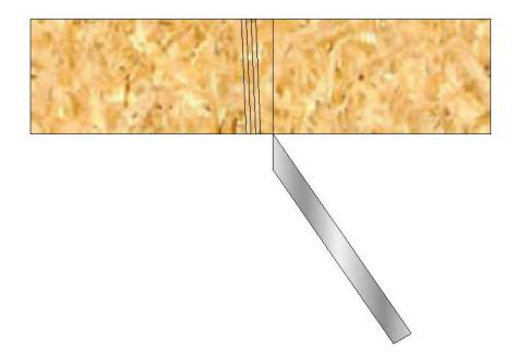
The next step is to push the cutting edge into the cylinder to make a "V" cut so you have a shoulder to ride the bevel against.
