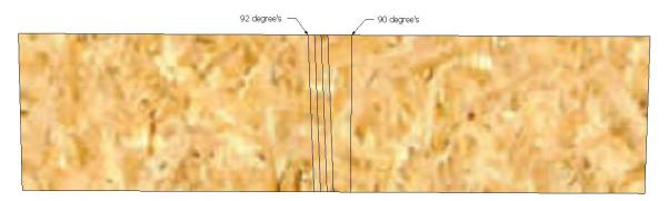
It is simple, if you present the tool at an angle, the tool will follow that angle. It is the same as cutting threads. The lines on the left are at a  $92^{\circ}$  angle or a  $2^{\circ}$  angle to the cylinder. The line on the right is at  $90^{\circ}$  or square with cylinder. The tool wants to follow the established lines, so a  $2^{\circ}$  will cause the tool to cut a  $2^{\circ}$  angle, spiraling around the cylinder.
