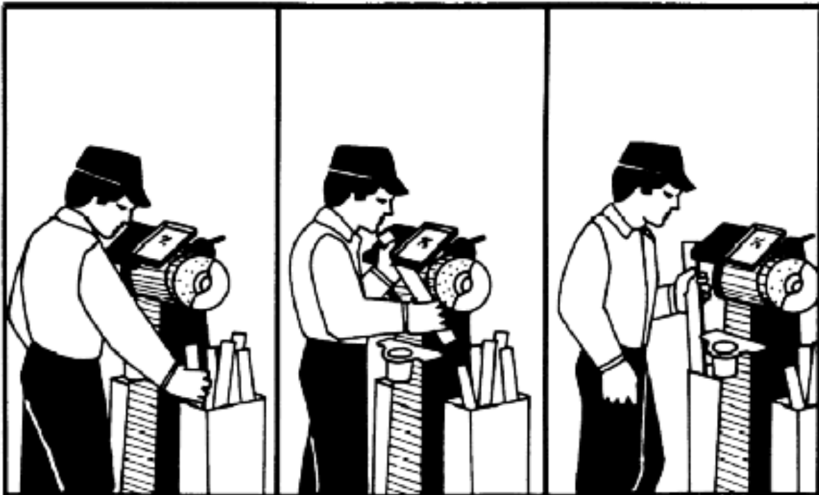
Figure 2. Grinding Castings: Hazards
