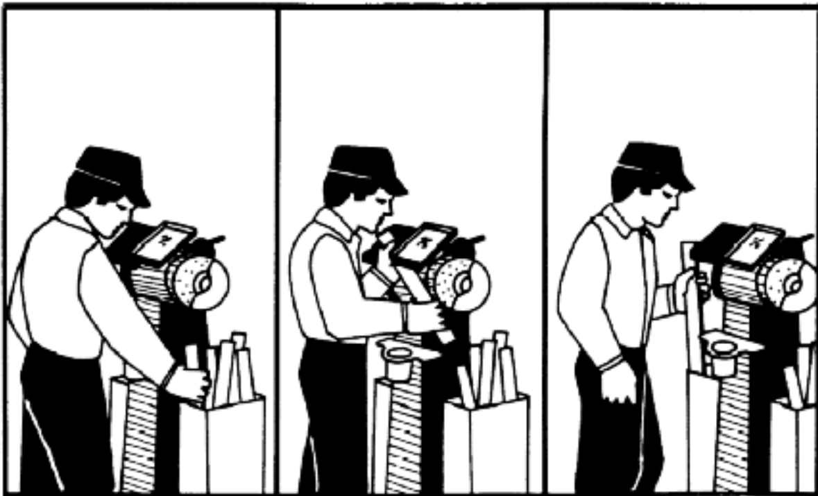
Figure 1. Grinding Castings: Job Steps
