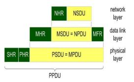
Fig.1: Structure of the IEEE 802.15.4/Zigbee frames
