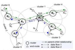
Fig.4: Cluster-tree topology with 2 time-bounded data flows
