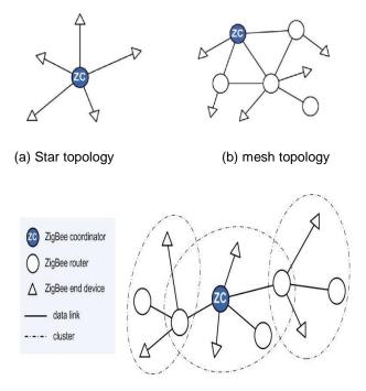
Fig.3: IEEE 802.15.4/Zigbee network topologies
