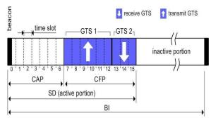
Fig.2: Super frame structure of IEEE 802.15.4.
